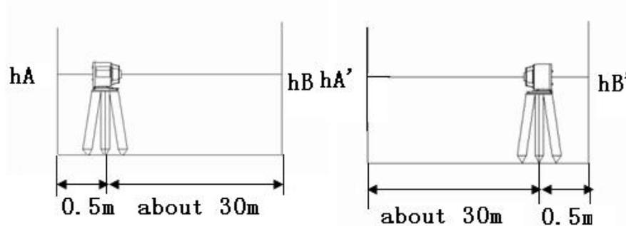
(2) Place the instrument according to horizontal setting and then adjust the instrument.
