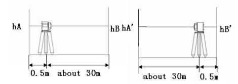
(2) Place the instrument according to horizontal setting and then adjust the instrument.(3)Switch on the power, and then measure the middle point of the laser beam on the
