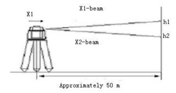
(2) After switching on the power, use the laser detector measuring the h1 of X1-beam on the wall or scaleplate.
