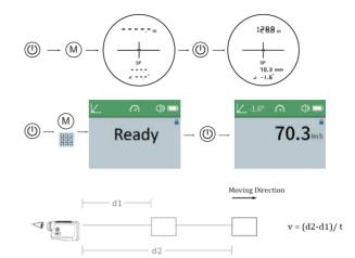
Speed mode can measure the speed of the target object moving in radial motion. The speed of the target object moving in parallel cannot be measured because the distance from rangefinder to target no change.
