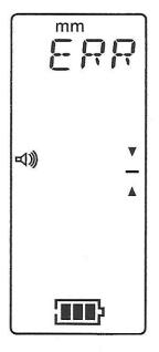
When Detector doesn't detect the laser beam, or laser beam is beyond receiving range, press SET key, the LCD will display ERROR and no further action.
